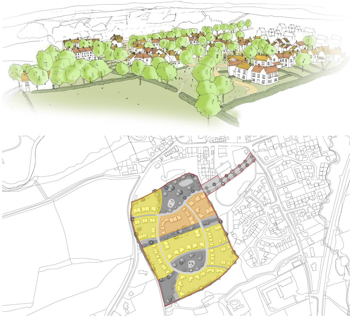
Figure 3.9: Two images from a neighbourhood plan masterplanning study – perspective to show how new housing in context (top) and building heights plan, indicated by different colours (bottom).
